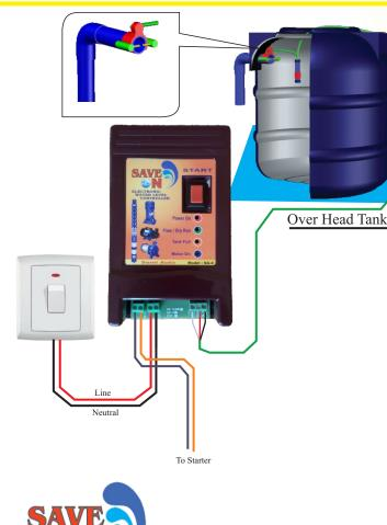
Connection Diagram of Semi Automatic Electronic Water Level Controller (SA-4) With STARTERS
